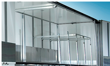
The EkeLoad beams allow for two-layer loading, also from the side.
