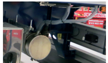
On the FNA and FRC products it's also possible to have a waste water tank with outlet valve.
