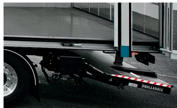
We are offering slider and cantilever tail lifts.
