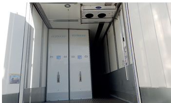
With an intermediate wall and 2-temp. cooling unit it's possible to divide the loading space into two compartments.
