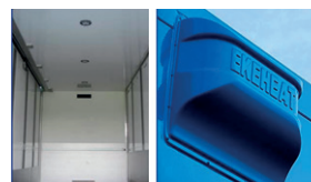
Ekeheat is Ekeri's own heater with air channels built inside the walls available in 5 kw, 8 kw and 11 kw versions
