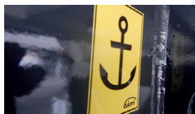
IMO A.581 -certificate ensures that 8 pcs of yellow marked ferry attachments are mounted on the chassis.
